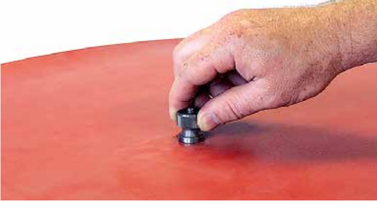
(Figure 5) Unscrew and remove the scale bar knurled nut from the scale bar assembly. Using the guide hole, position the gasket material onto the threaded scale bar spindle. Screw the knurled nut back onto the spindle to firmly secure the material. Hand tighten.
