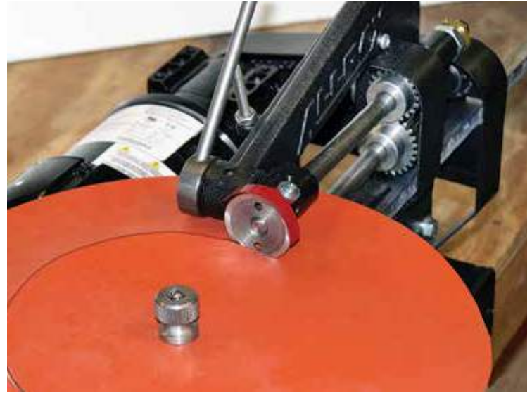
(Figure 8) To cut the inner diameter (ID), loosen the scale bar Tee screw, and slide the scale bar to the desired setting. Hand tighten the scale bar Tee screw. Engage the top cutting disc. Hold down momentary switch to engage motor, simultaneously maintaining downwards pressure on the cutting disc lever as before. Continue pressing switch until the entire ID of the gasket material has been cut. Disengage the top cutting disc and remove newly cut gasket. Unscrew and remove knurled nut from spindle. Discard unwanted material.
