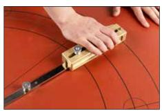
7. With slight downward pressure, rotate cutter block clockwise to make cut. Simultaneously press down on gasket material to prevent rotation.
