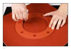
**1.** If existing gasket is available, using a pencil, trace outline onto gasket material.
