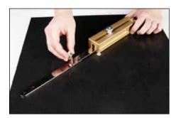
**5.** To cut gaskets over 25" (635 mm) diameter, add additional extension bar(s). Locate extension bar with threaded post and stud at one end. Insert threaded post and stud through dual holes at free end of installed extension bar. Secure with knurled nut.
