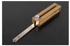
**4.** Gasket cutter can now cut up to 25" (635 mm) diameter. For example, to cut 16" (406 mm) OD gasket position pivot post indicator at 4" mark on large scale located on bottom of cutter block (12" + 4" = 16").
