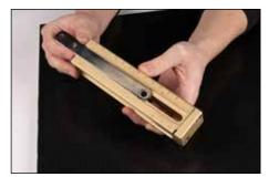
2. Locate extension bar without threaded post and stud. Orient extension bar with single hole nearest cutting blade. Slide extension bar into groove on bottom of cutter block.
