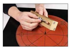
**13.** Loosen knurled nut. Slide pivot post indicator to desired ID. Tighten knurled nut. Repeat cutting steps.
