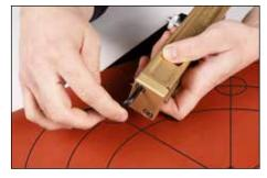
8 Loosen Allen screws on cutter block. Slide cutting blade into position. Position cutting blade to protrude slightly beyond thickness of gasket material. Tighten Allen screws.
