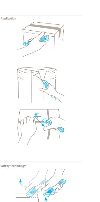
Automatic blade retraction – a high degree of safety The automatic blade retraction of the SECUNORM 300 guarantees a high degree of safety from cut injuries. As soon as you have started to cut, take your thumb off the slider. Then the blade will retract into the handle immediately after leaving the material being cut.
