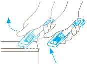
Automatic blade retraction – a high degree of safety The automatic blade retraction of the SECUNORM 300 guarantees a high degree of safety from cut injuries. As soon as you have started to cut, take your thumb off the slider. Then the blade will retract into the handle immediately after leaving the material being cut.
