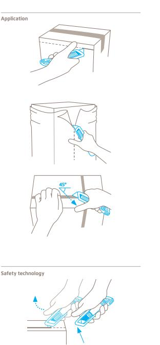
Automatic blade retraction – a high degree of safety The automatic blade retraction of the SECUNORM 300 guarantees a high degree of safety from cut injuries. As soon as you have started to cut, take your thumb off the slider. Then the blade will retract into the handle immediately after leaving the material being cut.
