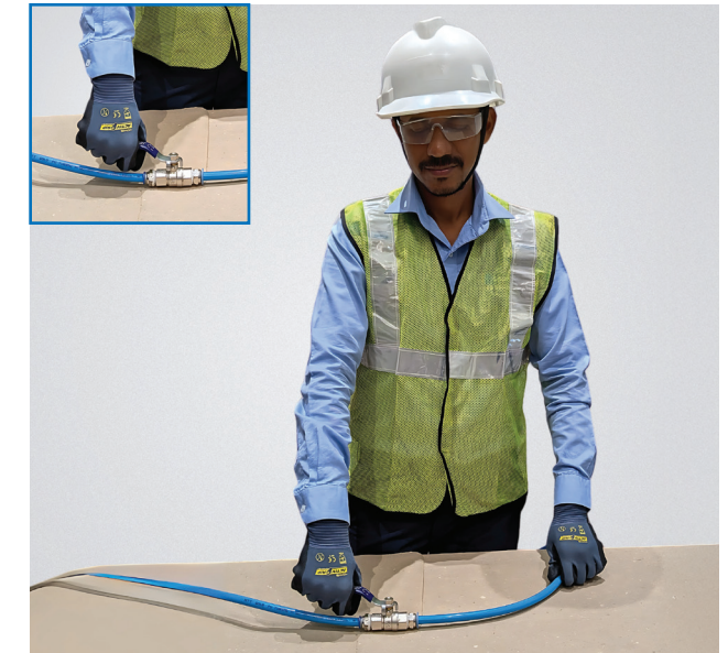
STEP 4 Open Air Valve - Slowly open the compressed air valve to allow air flow.
