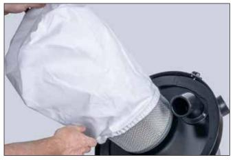
2. Remove the prefilter bag if needed. Regular prefilter bags slip over the filter and are secured in place with an elastic hem. PulseAir prefilter bags are secured in place with a wormgear clamp.
