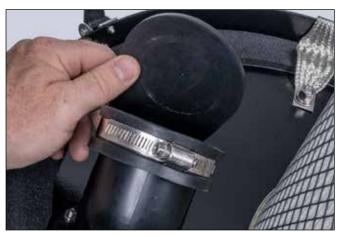
2. Inspect the reverse flow check valve. It should move freely. Replace if damaged, ripped or torn.
