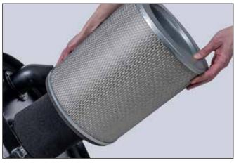
4. Lift the filter off the wire cage frame.
