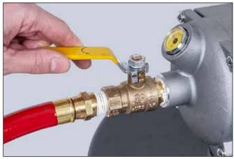
7. Open ball valve on vacuum to operate. Pressure gauge should read between 80 psi and 90 psi during operation for an optimally operating vacuum. If pressure is lower than 80 psi and the vacuum performance is inadequate, install lower flowing injector nozzles.
