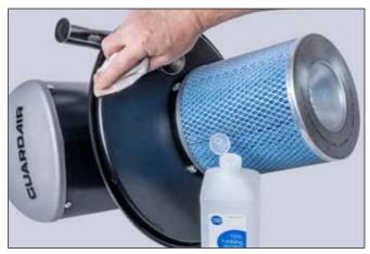
2. Hot Glue is the adhesive type used to bond the gasket to the vacuum cover. To remove dried residual glue, soak surface liberally with rubbing alcohol and allow to sit. Old glue should scrap off easily.
