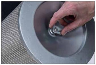
**3**. Remove the wingnut and sealing washers at the bottom of the filter.
