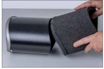
2. Remove the exhaust housing. Then remove the silencer foam.
