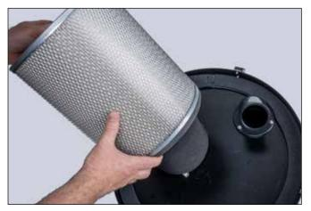
4. Lift the filter off the wire cage frame.
