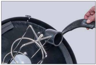
1. Remove the gasket to be replaced by hand.
