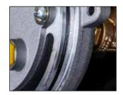
5. Inspect the o-ring on the manifold. Clean and apply o-ring lubrication if needed. Replace the o-ring if needed.
