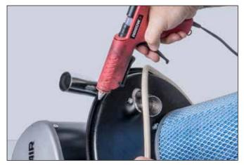
**3**. Use hot glue to install the new gasket. Lay the gasket in place and lift a starting spot to insert the hot glue nozzle.
