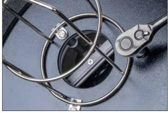
. Remove the three hex head bolts holding the PowerQUAD head to the cover.
