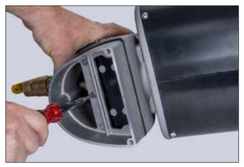
. Remove the 3 flat head screws securing the vacuum generating engine base.
