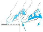
Automatic blade retraction – a high degree of safety The SECUNORM 610 XDR is equipped with automatic blade retraction: as soon as you release the lever, the blade disappears into the handle – and it stays there too. This provides a high degree of safety from cut injuries.
