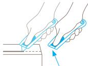
**Fully automatic blade retraction – a very high degree of safety** The fully automatic blade retraction of the SECUPRO MEGASAFE guarantees a very high degree of safety from cut injuries. The blade withdraws into the handle immediately after leaving the material being cut. Even if the slider is still being activated.
