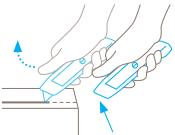
Automatic blade retraction – a high degree of safety The automatic blade retraction of the SECUNORM MULTISAFE guarantees a high degree of safety from cut injuries. As soon as you have started to cut, take your thumb off the slider. Then the blade will retract into the handle immediately after leaving the material being cut.
