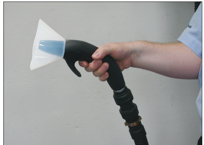
Chip guard attachment enhances operator safety
