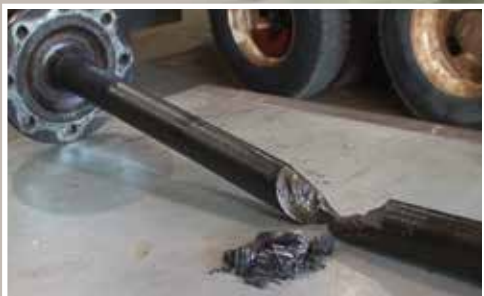
Broken axle with metal chips extracted from axle housing by the ReverseForce Air Gun .
