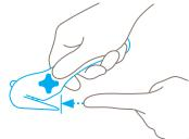
**Concealed blade – a maximum degree of safety** The SECUMAX COMBI blade is not an open one, but is hidden from people and goods. This provides you with the highest degree of safety from cut injuries and from damage to goods.
